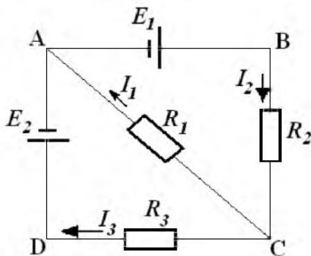
$$E_1 = I_1 R_1 + I_2 R_2 \quad -E_1 = I_1 R_1 + I_2 R_2 \quad -E_1 = I_1 R_1 - I_2 R_2 \quad E_1 = -I_1 R_1 - I_2 R_2$$
